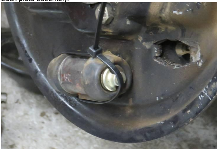
After taking off the brake drum, wheel hub and brake shoes, Mike put a cable tie around the pistons to retain them within the brake cylinder. We didn't want to disconnect the cylinder from the hydraulic system and have to bleed the brake cylinder afterwards. The copper hydraulic brake pipe was carefully unmounted from the axle. The brake cylinder was left attached to the brake back plate which was unbolted from the flange at the end of the axle and then carefully suspended on wire from a rebound strap mounting with the hydraulic pipe still attached.
