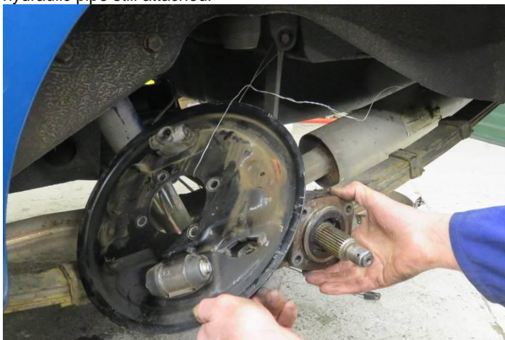
After taking off the brake drum, wheel hub and brake shoes, Mike put a cable tie around the pistons to retain them within the brake cylinder. We didn't want to disconnect the cylinder from the hydraulic system and have to bleed the brake cylinder afterwards. The copper hydraulic brake pipe was carefully unmounted from the axle. The brake cylinder was left attached to the brake back plate which was unbolted from the flange at the end of the axle and then carefully suspended on wire from a rebound strap mounting with the hydraulic pipe still attached.
