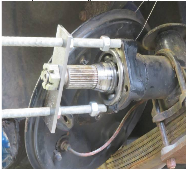
By tightening up the hub shaft nut, the half-shaft should come out.
