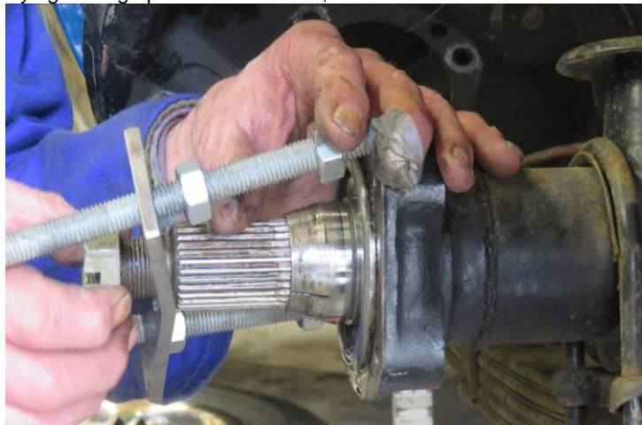
Oh dear, the plate has bent - it wasn't strong enough! On to half shaft pulling tool Mark 2.
