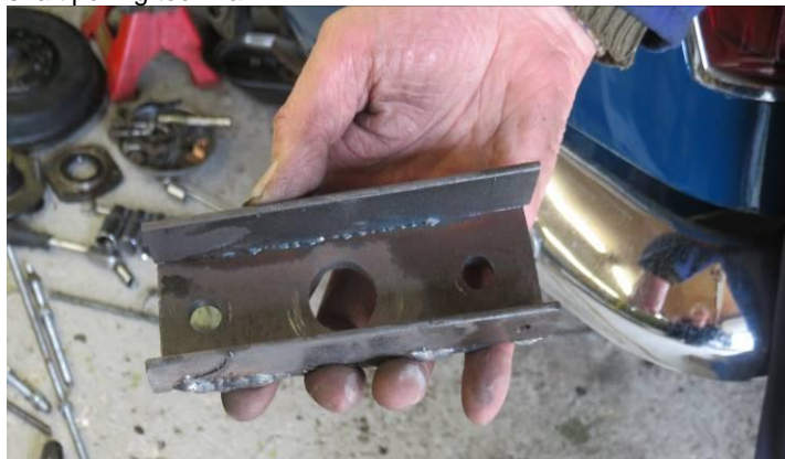
Mike straightened out the plate and strengthened it by welding on a couple of side flanges.
