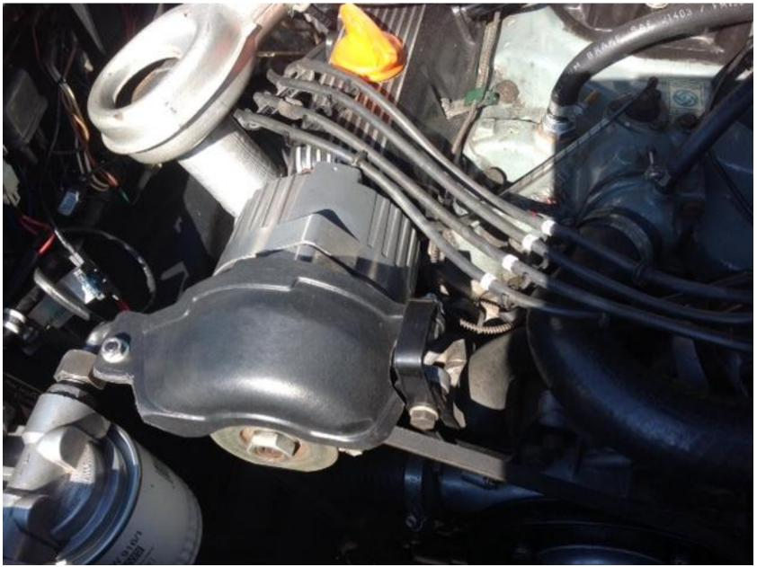
An alternator cover seen on a late rubber bumper MGBGTV8 in Switzerland. Victor Rodrigues thinks "it is a good idea providing efficient safety when doing some inspection or repairs whenever the engine runs. Do you know if this item was a standard/factory BL equipment or a simple after market item? Do you know if it is still available to purchase?"
