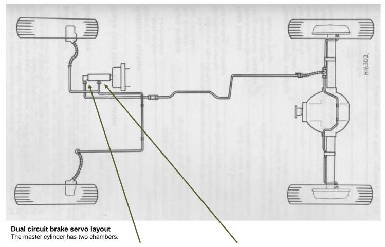
**Front chamber** feeds the <u>rear</u> <u>brakes</u> with a single pipe.
