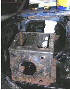
twinned outlets, and the rear brakes to the second stage outlet. This way if one circuit fails I should still have either front or rear brakes working (see photo).
