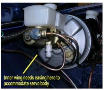
Hydraulic brake layout, later type (RH drive) with tandem master cylinder and servo.
