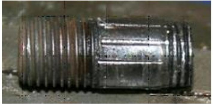
Setting it to run anticlockwise the impact wrench screwed the remainder of the stud out of its hole in about 15 seconds, the length of time showing how tightly it was held by the rust of the ages. It is possible to use a ½" drive bar but this might not be as easy as using an impact wrench, unless you have a very long one and the space to manoeuvre it.
