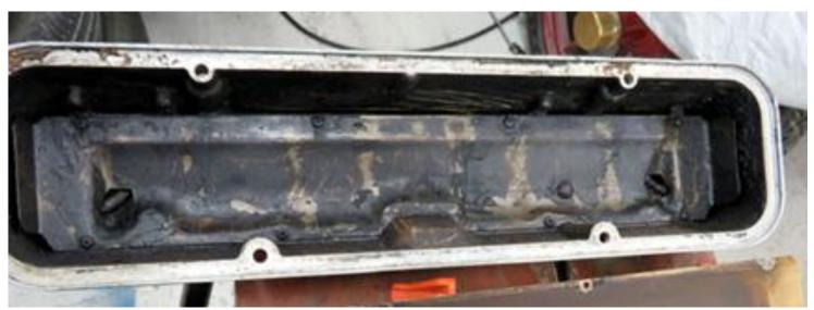
Another rocker cover amongst the spare bits that came with the MGBV8 Roadster conversion. This shows you the build-up of muck on the inside of a high mileage Rover V8 engine.
