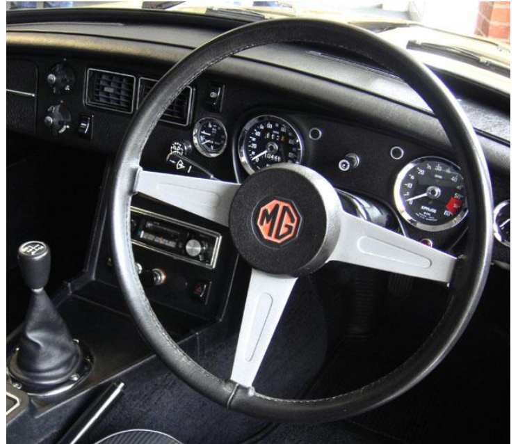
Horn push on an earlier MGBGT V8
