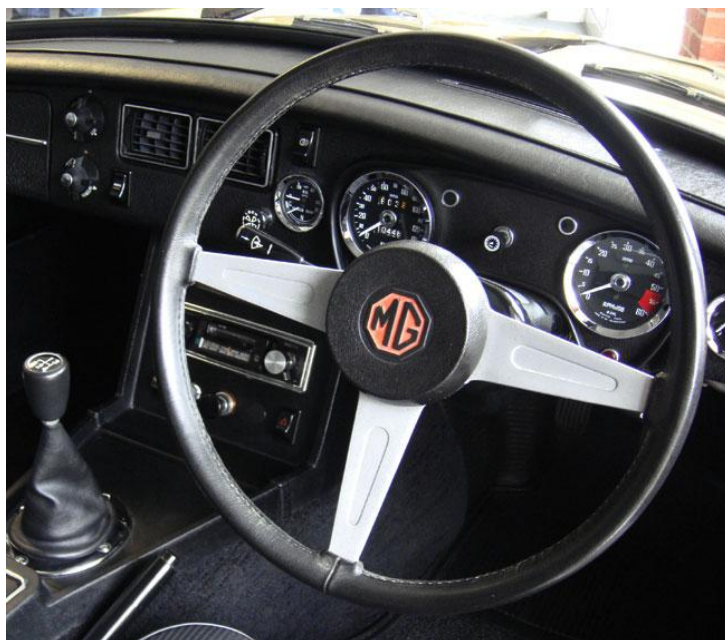
Horn push on an earlier MGBGT V8
