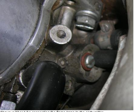
Above: rubber tube connecting the flame traps to the carburettor
