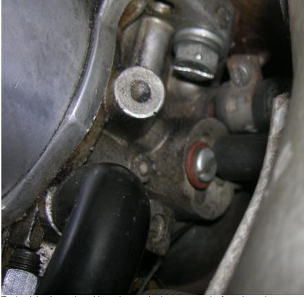
To the right above, the rubber tube attached to a vent outlet from the carburettor – the tube then runs round the back of the carburettor air box and down to the "T" piece.
