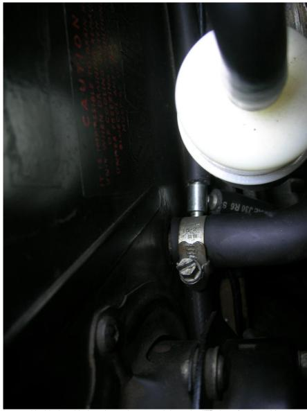
Located behind and below the carburettor air box, the "T" piece for the rubber tubes venting each carburettor and, connecting to the lower end of the "T" piece, a third rubber tube which takes any petrol that might overflow down low so it is released away from the hot exhaust. The "T" piece is not easy to see and harder to get at.
