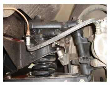
The effect of a hose with both ends an extra 8mm long would be to reduce the flexible portion by 16mm compared with a genuine Lockheed hose. If the flexible part is not long enough then there is a possibility that the hose may be overstretched when the steering is on full lock, which could possibly lead to premature failure of the hose.
