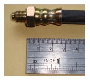
I have measured new rubber hoses from five different manufacturers - Moprod, Veco, Brovex, Classic Gold and a genuine Lockheed hose. What is immediately apparent is that the length of the crimped metal ends varies quite a bit. The original Lockheed hose had metal ends 25mm long (excluding the threaded portion). The others had 27, 30, 32 and 33mm ends.
