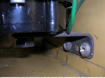
**Next unscrew the bolts securing the horn bracket** to the bodywork on the side of the space behind the grille (see above).
