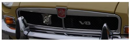
**Refix the grille surround** starting with the three bolts along the bottom of the grille and then the three top bolts on the top edge of the grille surround. Before tightening up ensure the grille is centred in the grille opening so the gaps are even all round.
