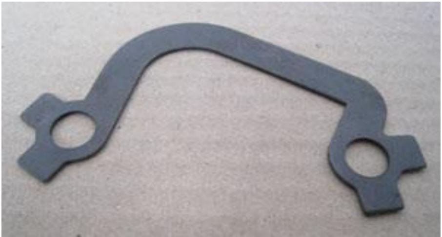
**John Brown** posted a note on the V8BB saying "just experienced loose exhaust manifold studs on the top two rear left hand side studs. A 14mm A/F socket fits in various combinations to get to at most of the others. Access to the rest would be from underneath. Why aren't these studs fitted with anti-vibration washers? Studs with a flat washer do not seem like a good solution. Maybe we can improve on this with a special washer."
