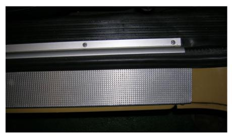
**Left**: view from passenger legwell to the door seal sill retaining strip showing it has a profile like a number **2**.
