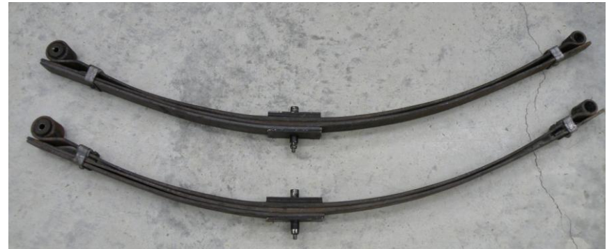
General view of repaired springs with extra "half leaf" on the "front" part (LHS above) of the spring
