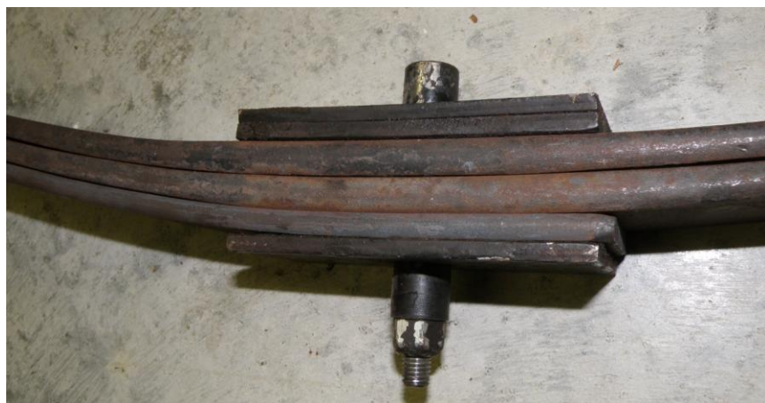
Shows half leaf (centre mount forwards to front spring eye) - one "spacer" removed to allow for the third leaf
