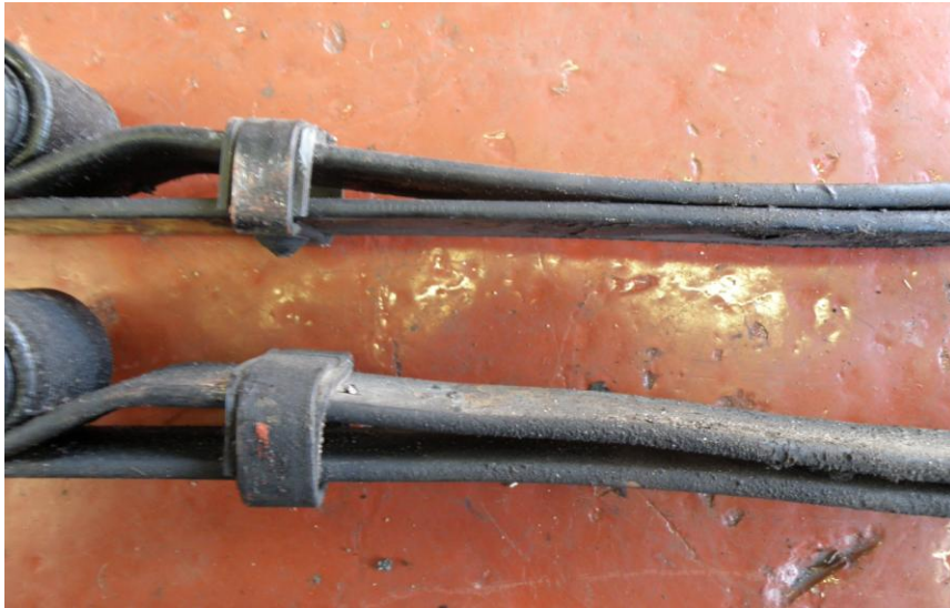
Upper spring as it should be –lower spring is bent due to torque
