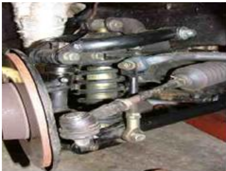
Front suspension with the coilover damper conversion (Photo: Geoff King)
