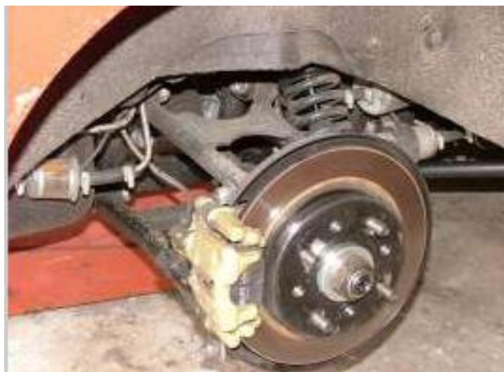
Rear suspension and disc brake conversion. (Photo: Geoff King)
