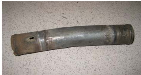
Steel pipe connecting the two lower cooling hoses is badly corroded with a hole. (Photo: John Holmes)
