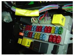
Wipers failed? – test the relay as well as the fuse
