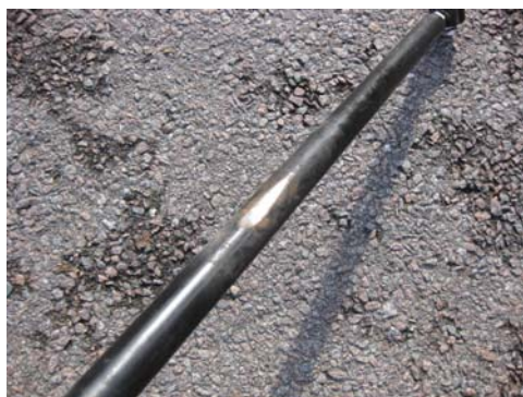
Panhard rod polished from friction contact with the diff casing. (Photo: Angus Munro)
