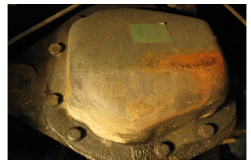
Differential with the impact marks from the Panhard rod: a long mark to the right and a spot mark which was shiny two months earlier. (Photo: Angus Munro)
