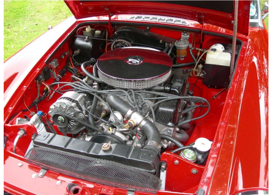
An electronic temperature sensor for cooling fans is located in the top hose.
