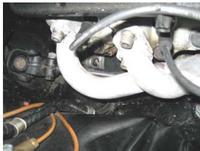
Shows the upper starter motor bolt, centre of picture with the screwdriver slot shown in white. Note the proximity of the upper column.
