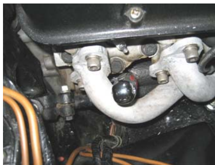
This shot shows the ratchet handle in position with socket engaged. The handle is at the bottom of its travel, and can move up almost as far as the spark plug electrode.
