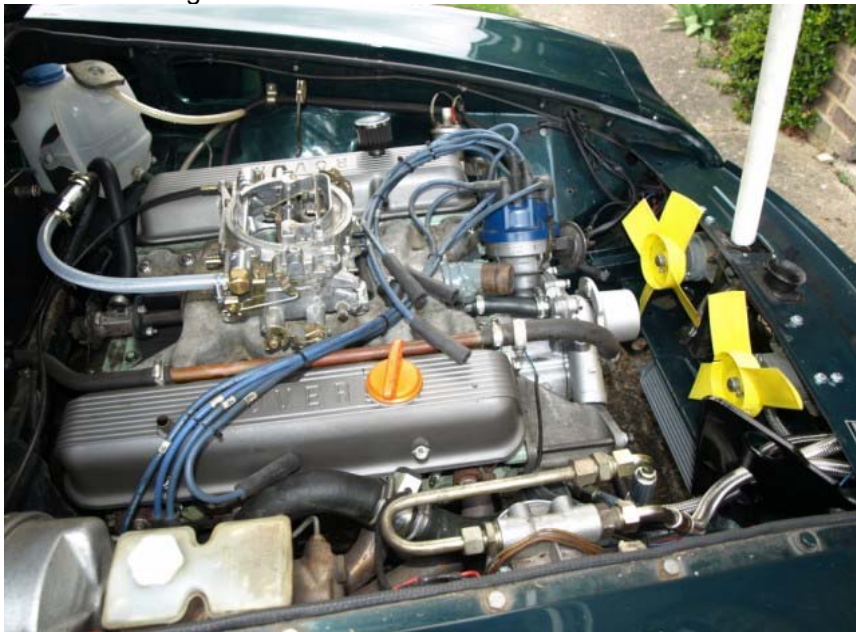
SD1 3.5 V8 engine with stainless steel RV8 tubular exhausts through the inner wings
