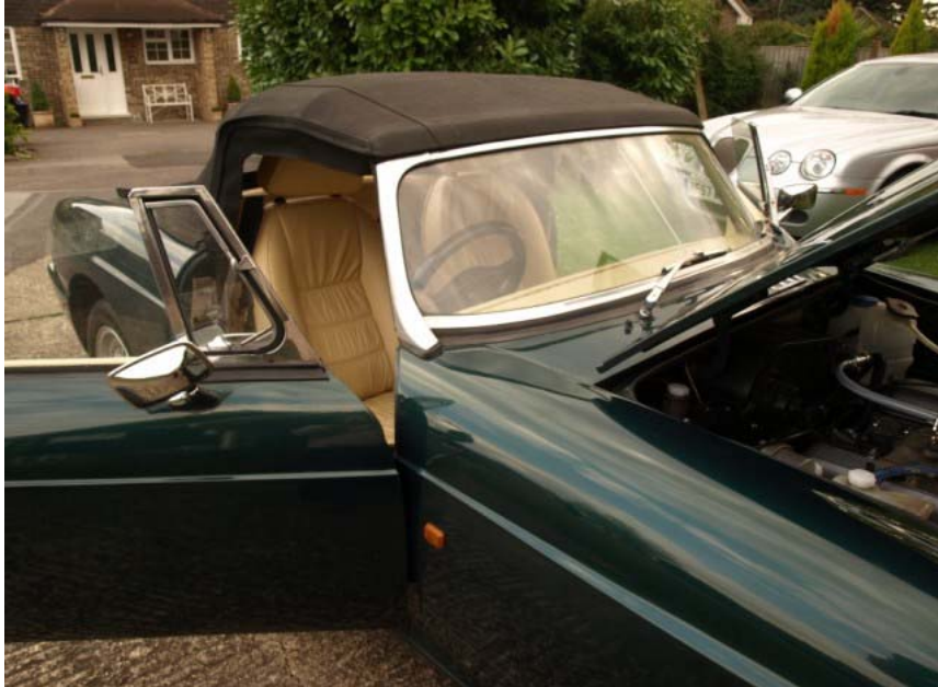
MGB alloy windscreen frame so no RV8 windscreen rusting problems, and door quarter lights are fitted
