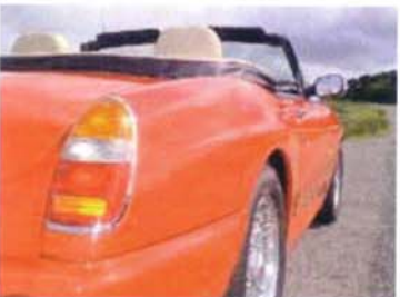
The cleverly fashioned bumpers in the body colour suit the flowing lines of the car – note the rear light cluster, another item that was different to the part on the earlier V8 model. (Photos: Bill Wood)
