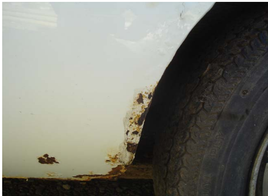
Lower section of the nearside sill and lower rear wing
