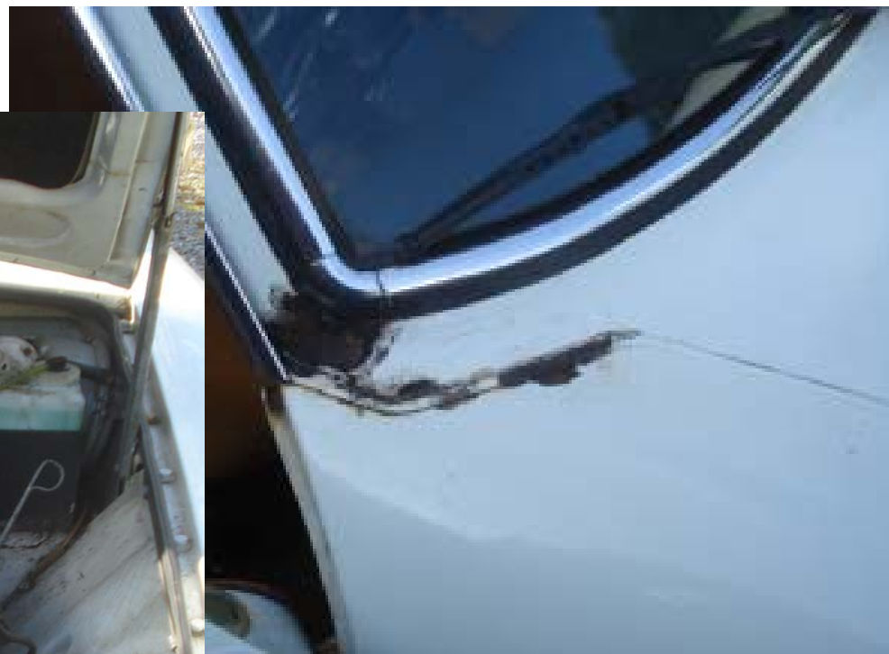
Offside dogleg joint between the wing panel and main shell and windscreen
