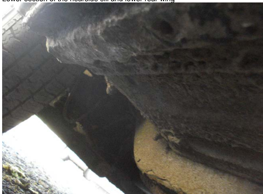
Underside of the nearside sill coated in underseal
