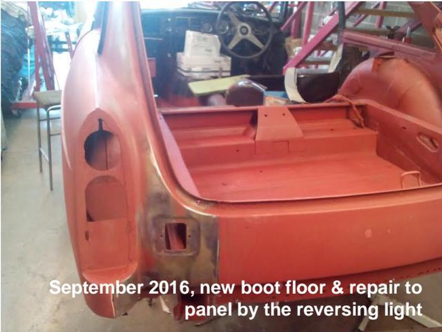
September 2016, new boot floor & repair to panel by the reversing light
