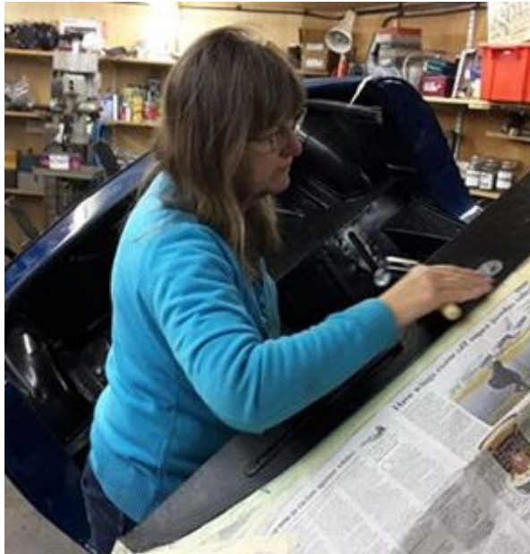
Jane using a roller on the vinyl trim on the scuttle panel
