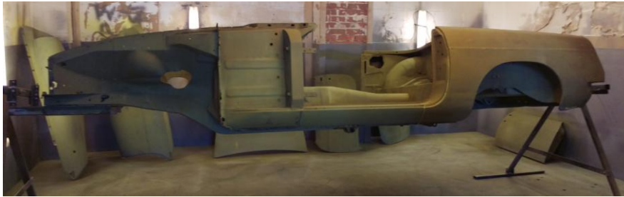
The bodyshell etch primed to stop the clean metal going rusty.
