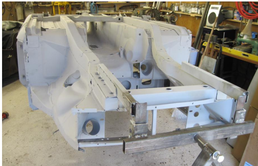
The bodyshell mounted on the spit and turned upside down. Just to prove the shell does rotate easily.
