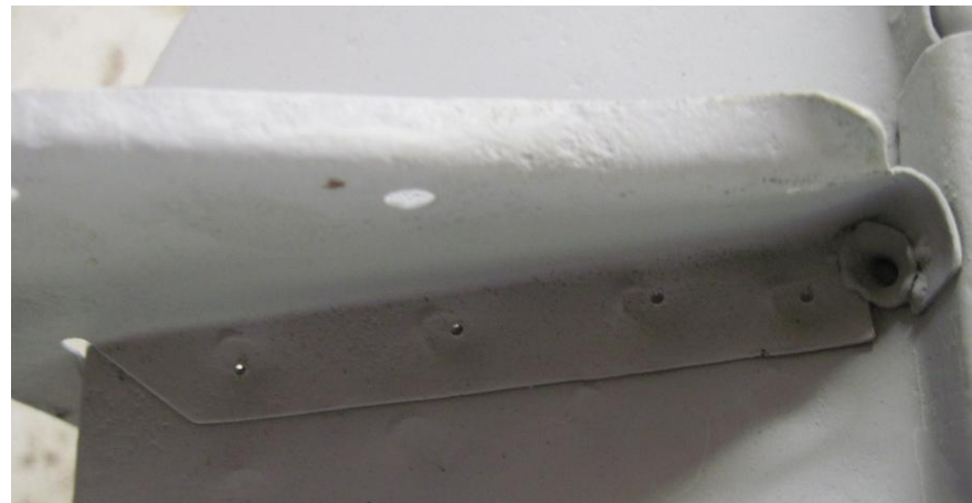
OK, let's get down to some work. Centre punch the spot welds.
