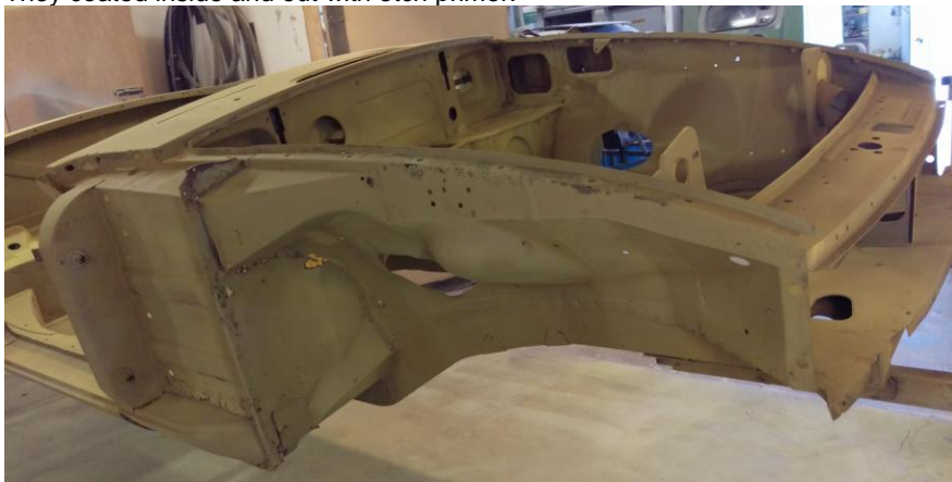
The bare bones of the bodyshell. SBL, blasted, etch primed the two doors, both front wings, bonnet and boot lid. I asked them to etch prime the shell so that it would not start to go rusty. They also, free of charge, painted the shell in 2-pack primer as they said "It came in yellow; we did not want it to go back yellow!"
