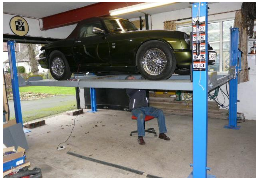
Raised 1200mm , best for all major work underneath. Highest I can go under the beam.
