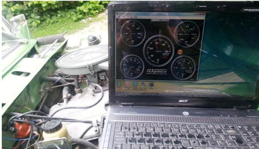
Ignition advance shown on the screen in real time with the engine running. Turn off the ignition; connect the black wire to the coil. Start the engine. This was no problem at all – it started first go. Pete then connected the laptop to the USB
