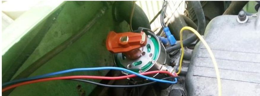
Turn on the ignition, rotate the distributor until the little green light inside the distributor comes on. This was a little difficult to see, probably due to the bright sunshine.
