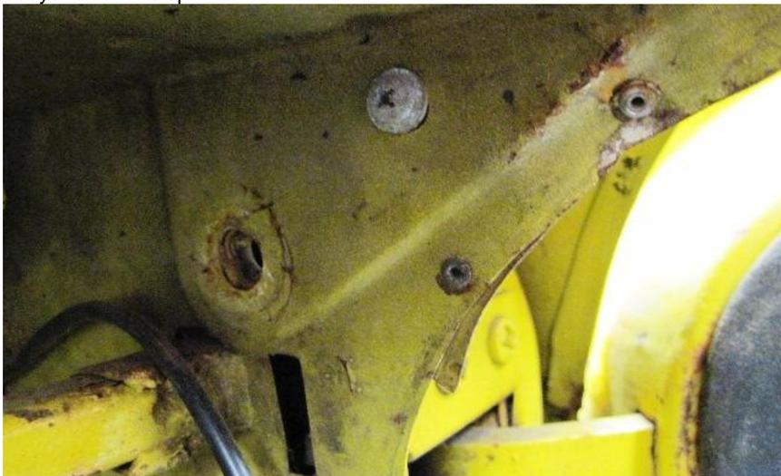
Both the striker and the lock were cleaned up with some WD40 to help the fixing screws come out and clean off the years of grease and muck that accumulated on them.
