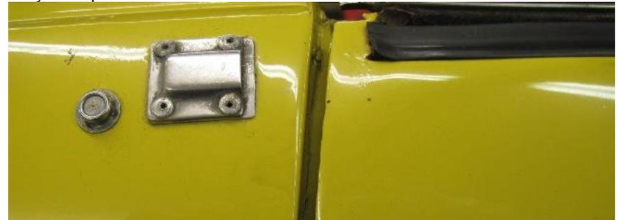
One of the items was to adjust the doors so that they opened and closed nicely. As you can see from the photo above the door is slightly down from the rear wing
