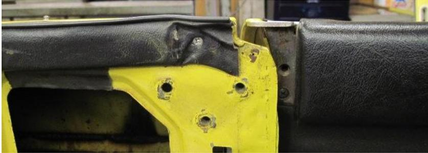
The mounting point for the hood frame which will do for fixing the door aperture brace on the 'B' post.
