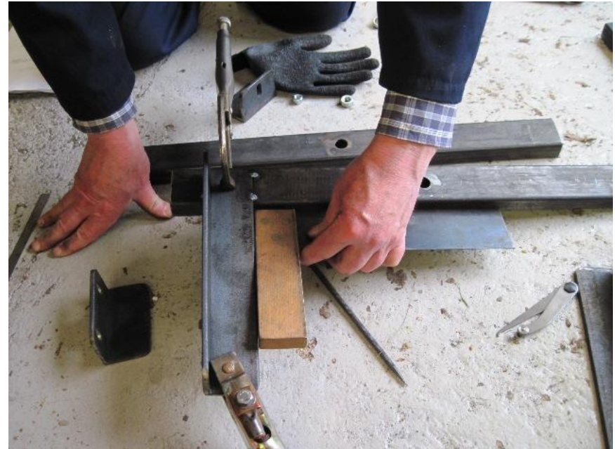
Dugald checking that the parts have been tacked at right angles with a square.
