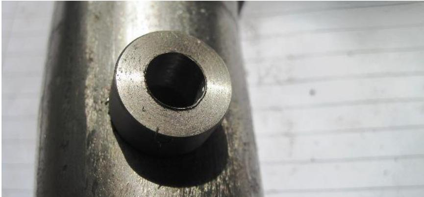
It would be great if the M12 x 1.25mm tap arrived in the post today so I can thread the oxygen sensor in the lathe before I take the parts down to Freewheel to TIG weld the collars on. I don't want to have the collars welded on first before tapping the thread as it will be difficult to hold the tap wrench square. Also the upper part of the downpipe will get in the way of the tap wrench. I have just thought of another tip.
