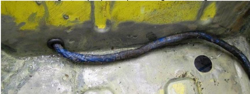
Hole cut through the side of the sheet metal where the battery is located.
