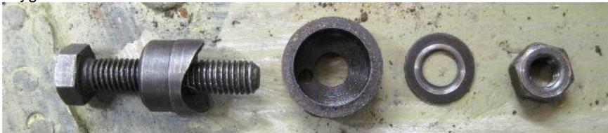
At last I have made a decision and decided to run the battery cable and the electrical cables to the rear of the car inside the car. These hole punches are very useful for cutting holes in sheet metal.
