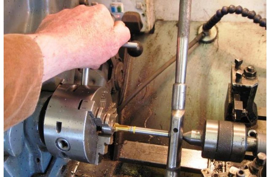
Once the thread has started I fit the tap wrench to the tap and fit a rotating point in to hold the tap square with the collar and finish the thread by hand.
