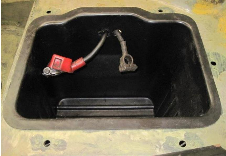
The battery box in place with the holes for the cables cut through both the battery box and the sheet metal. I may need to obtain or make a longer battery earth lead. It may be just long enough. I ran out of energy to do anymore today and had a little sleep this afternoon after my Cromer Crab lunch, which was very tasty and a treat.
