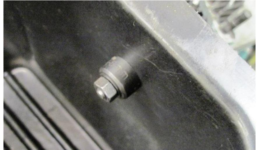
To find the position for the hole in the plastic battery box, I fitted the battery box in place and scribed through the holes in the metal to the plastic box from underneath the car. Took the battery box back out and cut the hole in the plastic with the same sheet metal cutter. I have just thought – I think these cutters maybe called 'Tank Cutters', but I may be wrong.
