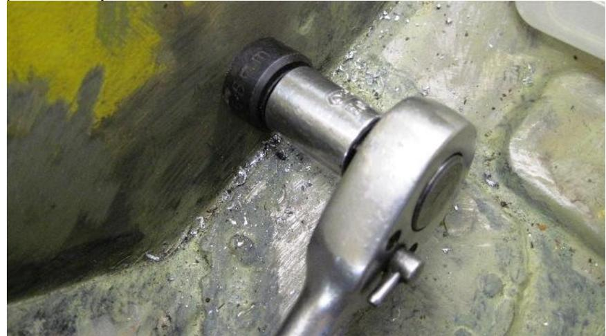
You drill a hole, that the bolt of the cutter will go through, then put the bolt with one half of the cutter on one side and the other side of the cutter and nut on the other side. Tighten up the nut with a spanner or socket and 'Bob's your Uncle' you have a neat hole for your rubber grommet and cables.
