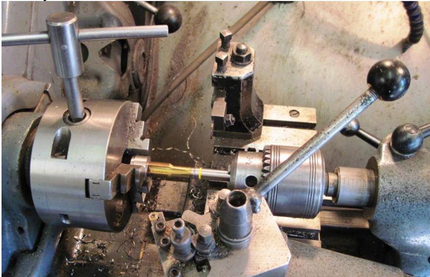
Tapping the thread for the oxygen sensor collars in the lathe. The tap in the drill chuck is locked and does not turn. The chuck in the lathe is rotated to start the thread cutting in the oxygen sensor collar. I rotate the lathe chuck by means of the chuck key.
