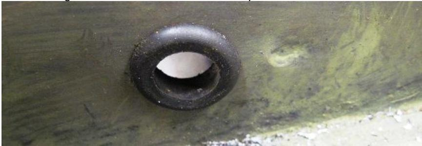
The cable for the lights, fuel pump etc. in place through the rubber grommet.
