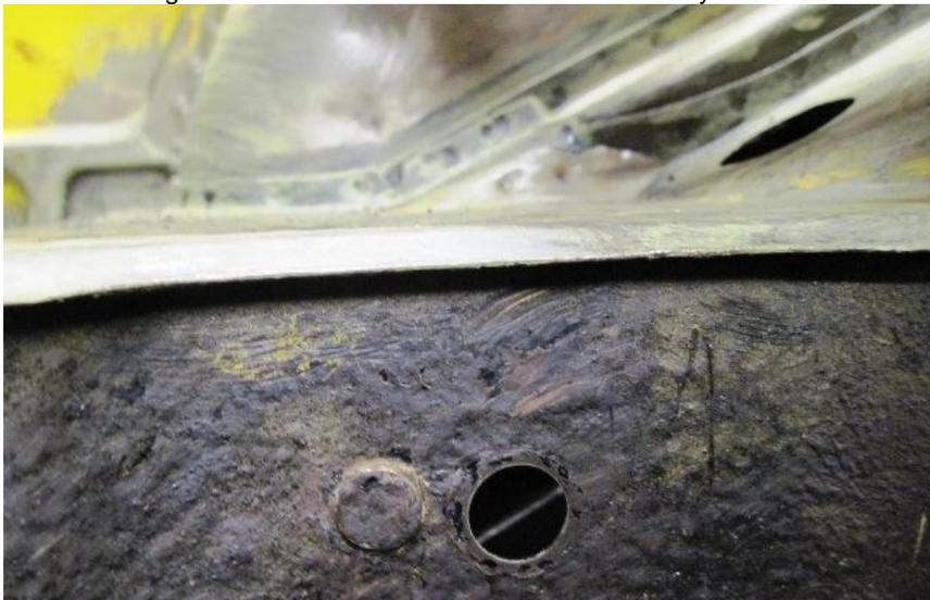
The way I marked the position of this hole was to fit the plastic battery box, put in the battery and measure the approximate position of where I wanted the hole.
