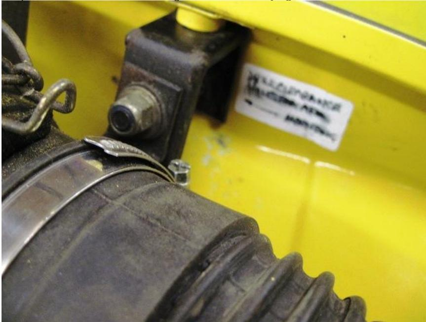
I bolted in the air mass meter to the bolt on the wing, to inner wing join. I need to drill another hole in the inner wing for the other mounting bolt. I scribed where the hole is to go and made myself a sticky label to put on the inner wing to remind me when the engine comes out. No it's not a shaky photo - the ink wasn't dry on the sticker when I stuck it on to the inner wing and the writing smeared – we can all make mistakes!
