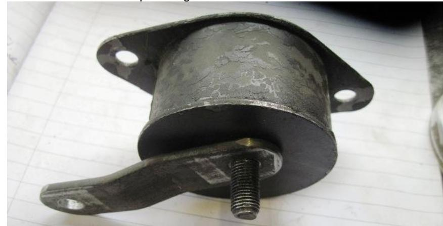
The rear engine mounting nearly ready to help the front two engine mountings deal with the torque from the RV8 engine.
