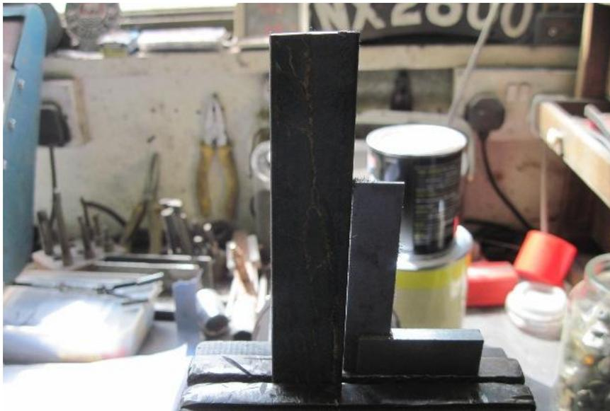
When you are going to bend a bit of metal in the vice it is an idea to put an engineer's square next to it to check you have the metal at right angles to the vice.
