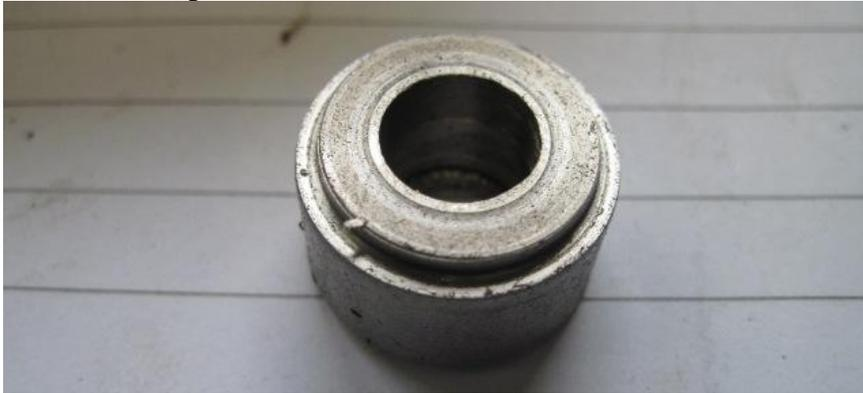
I should have made it a bit cleaner for the photo! I cannot put the thread in yet as I have not got a M12 x 1.25mm tap. I ordered one from e-bay. Although I normally buy drills and taps and dies of Tracy Tools 01803 328603 [info@tracytools.com](mailto:info@tracytools.com)
