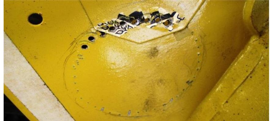
Instead of drilling straight away with a 4mm drill I started each hole with a 3mm drill instead. I just tried the top bit with the 4mm drill to see if my plan would work.
