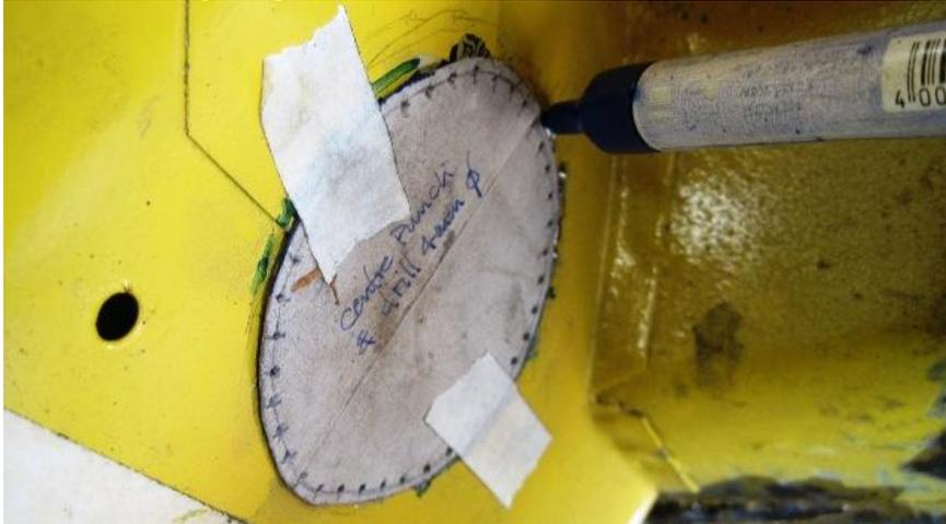
I checked the collar in the hole and of course it would not fit as the jagged bits of metal would be in the way. Stick back the cardboard template and draw around it with a felt pen to give me an idea of how much metal to grind away.
