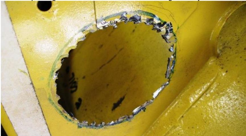
Now I changed the small cutting disc for a tiny milling type cutter that would fit in the Dremel. I keep calling it a Dremel, but mine is made by Clarke. I suppose it is like calling a vacuum cleaner a Hoover, or are they now all called Dysons? I originally bought one of these tools to clean up the welding when I had to repair the 1899 alloy wheel for the Perks & Birch motorwheel that is another project!
