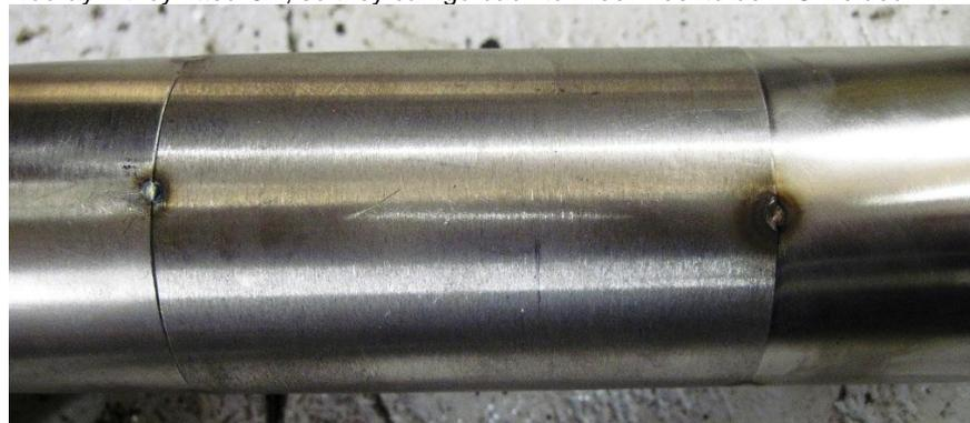
I wish I could tack weld like this with a TIG welder. The problem is that the amount of work that I have that needs TIG welding does not warrant me buying a set. Next I got on with making up the pipe to go through the LH front radiator panel for the air intake pipe and air filter for the engine.
