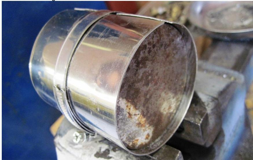
With the bent stainless steel sheet clamped on the mandrel I carefully panel beat the metal into the ring or I suppose you should call it a collar.
