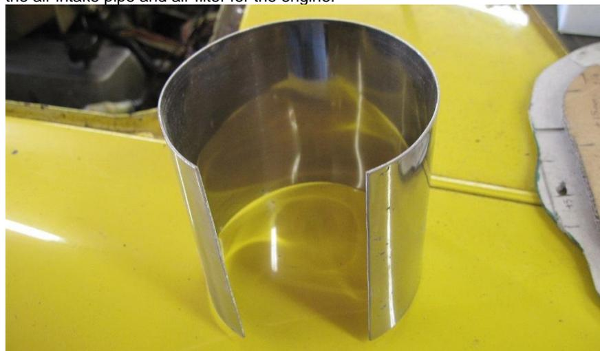
I had the stainless steel sheet rolled by Freewheel into a 3" diameter tube. They could not get it perfect on their set of rolls so a bit of panel beating was needed. I found a scrap of 3" diameter bar in my workshop and used this as a mandrel to beat the edges to shape on. First I fitted a worm drive clip to hold it in position on the 3" bar.
