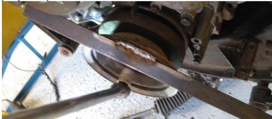
Then I could use a ½" drive socket with a breaker bar. Still no joy, I had to resort to a length of scaffold bar over the breaker bar, success. With the bolt removed I removed the rest of the crank pulley (damper).
