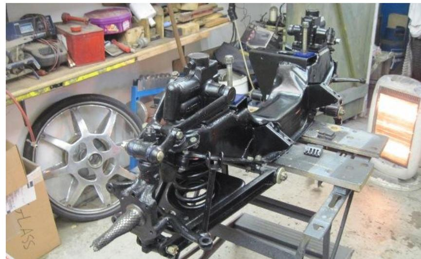
The front suspension assembly from Dugald's factory, V8 nearly ready to fit to the car.
