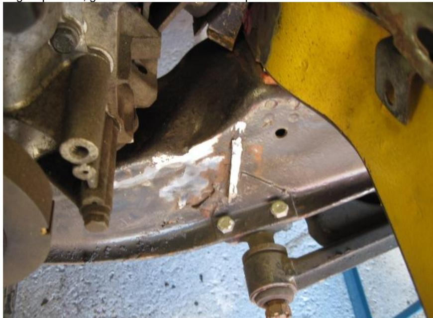
RH steering rack mounting nearly cut off and the welds ground down.
