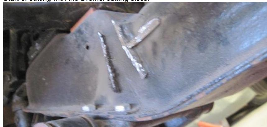
Successfully cut off with only using two of the small 38mm cutting discs. I did not cut closer to the front crossmember as I thought I would use less cutting discs. I
