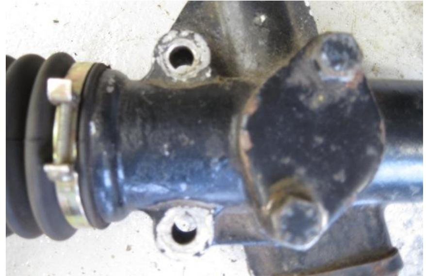
Getting gearbox mountings off is going to be a pain due to being cut off. Trying to get the rest of the mounting off the gearbox is not easy as there is nothing to hold on to. May need a centre punch and hammer
