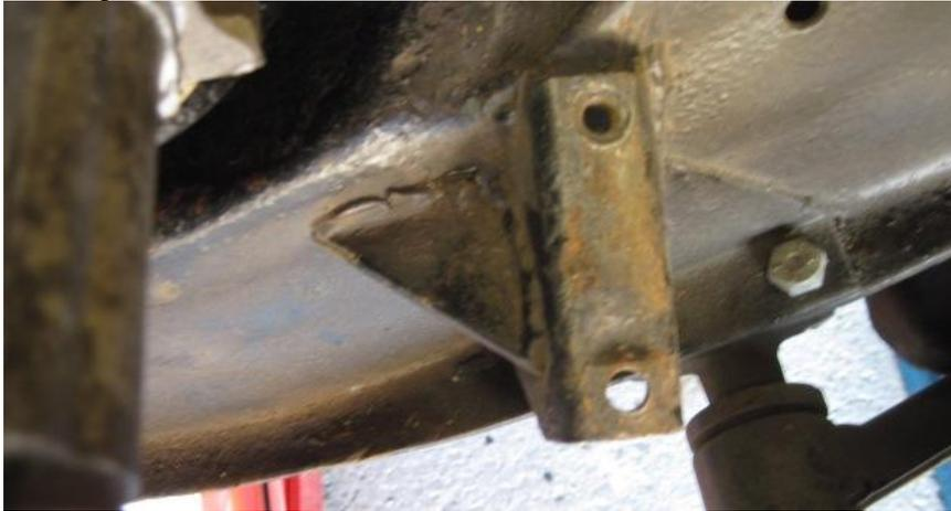
If I am to use this steering rack those elongated holes will have to be drilled out in the pedestal drill and stainless steel sleeves inserted to bring the diameter for the bolts back to original. I can make these in the lathe.
