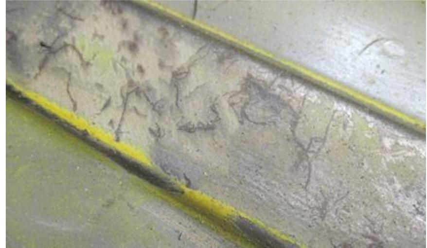
Sure enough under the paint were the **rust spiders**. Next I used the reversible drill with the "mule skinner" attached to grind out the rust spiders.
