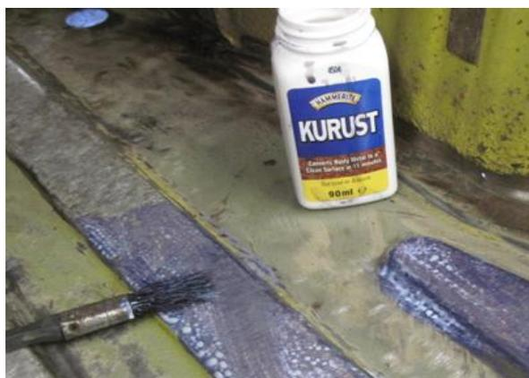
Next a thin coat of **Kurust** to stop any of the rust spreading. Leave the Kurust for a few hours and it will turn the metal black. It can then be coated in etching primer for even more protection.
