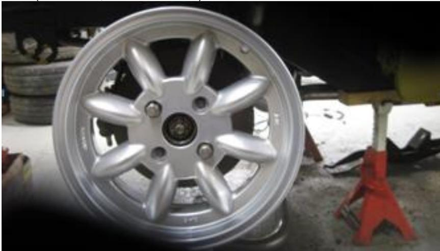
Normally if you fit wider wheels to a vehicle you have to make sure that the inset/offset is correct so that it adds the same distance to the inside and outside of the wheel rim so that the effective king pin angle bisects the tyre contact patch in the centre of the tread
