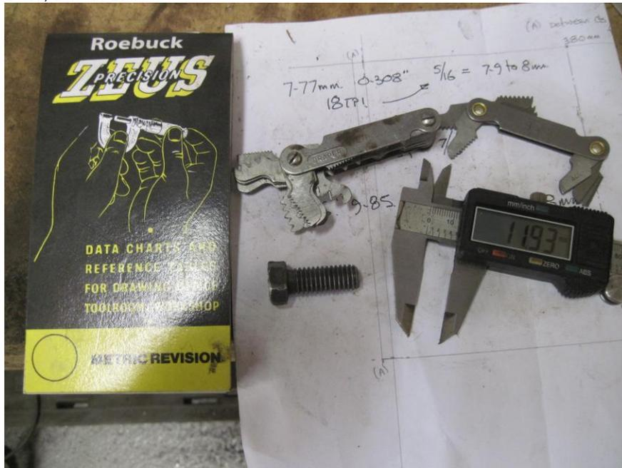
This shows a vernier calliper, Thread gauges for UNF, UNC, Metric and Whitworth threads.
