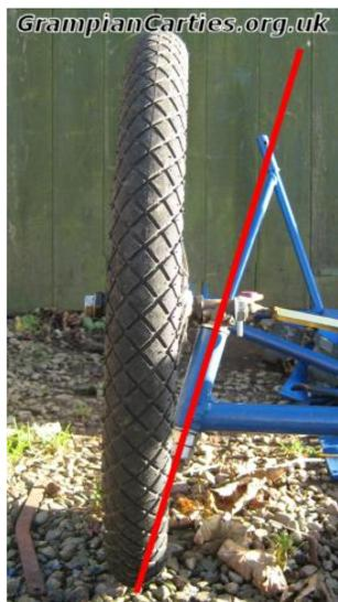
When I got the wheel and tyre home I tried it on the MG to make sure everything fitted OK and it didn't foul anything. I also added the height and width of the tyre to my drawing. Then I extended the line of the king pin down to the tyre. Low and behold it dissected the tyre contact patch right in the middle – perfect. Was it luck by the last owner, or well designed?
