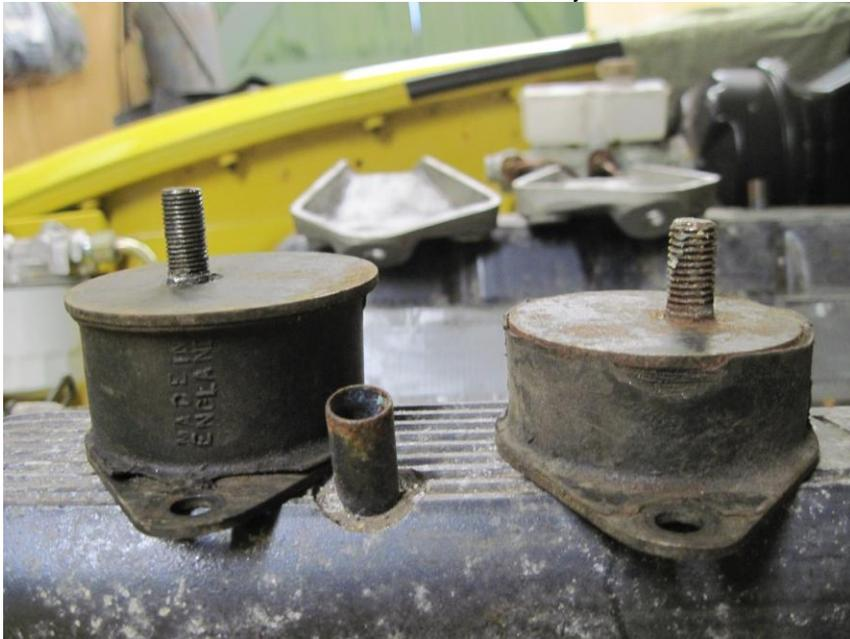
Engine mounting rubbers that were fitted to the V8 engine.
