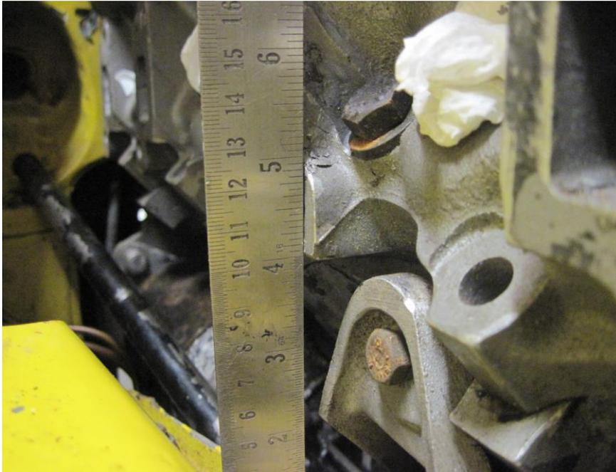
**Left:** checking the height of the top of the engine mounting bracket above the chassis rail. There is a photo of the other side that shows they are the same measurement, but I must have had the shakes when I took the photo
