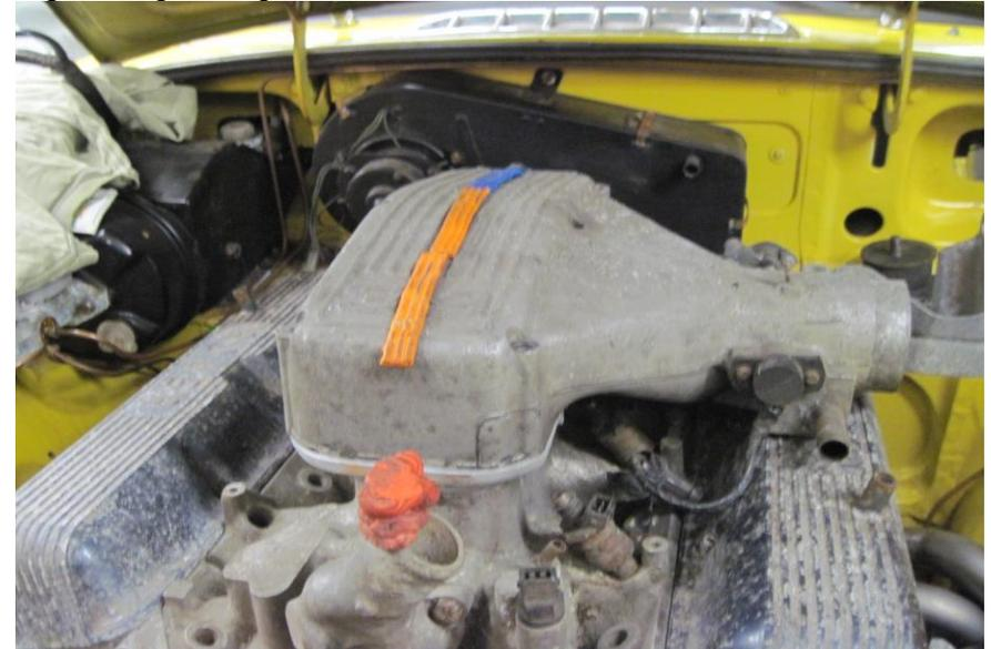
Checking with plasticine that the EFi bits will fit under the bonnet. They do at the moment, but I will check again when the new engine mounts are in place.
