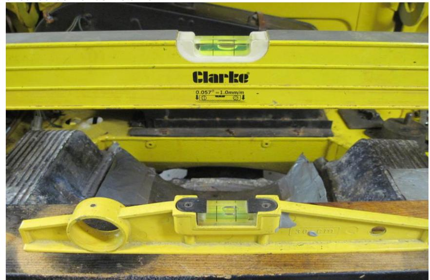
Checking that the engine is level with the tops of the wings.
