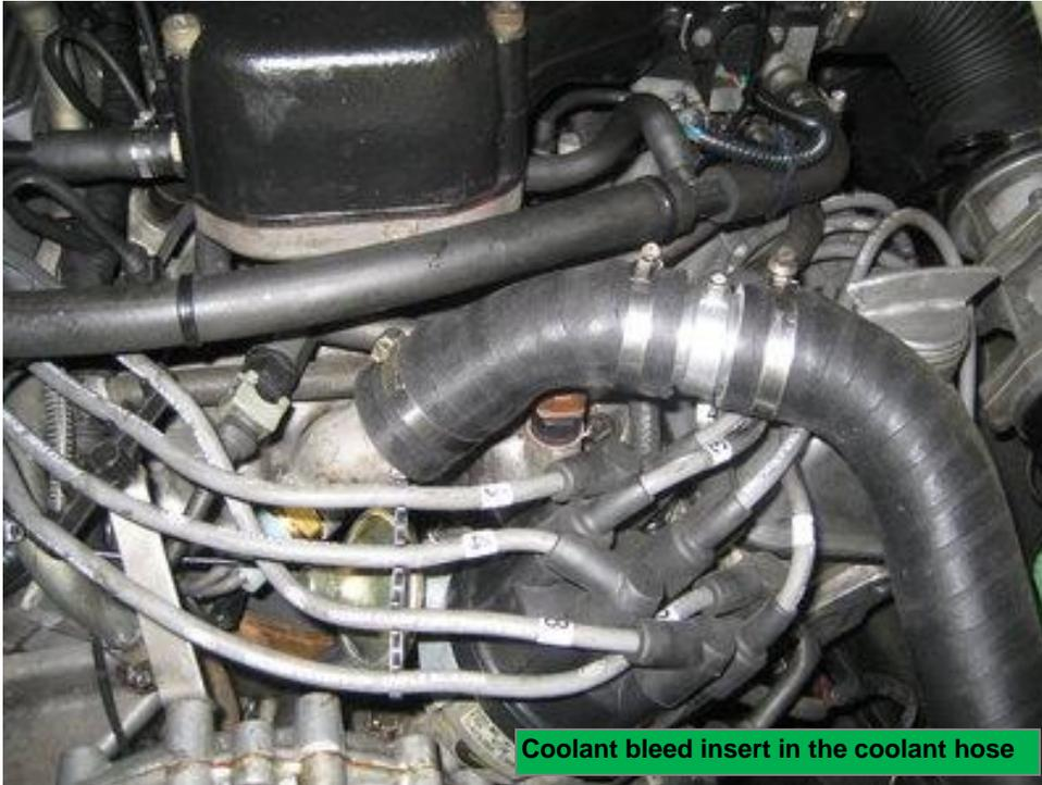
Coolant bleed insert in the coolant hose
