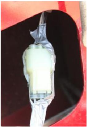
for mounting just the control knob it was fitted by the right hand door pillar to avoid it being near to the drivers left knee. Fitting used an existing hole in the car metalwork but did need a hole to be drilled through the inside trim. The bracket was coved in leatherette matching the RV8 trim.
