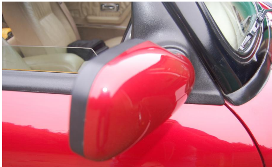
Electrically operated MGF wing mirror fitted as a replacement to an RV8.
