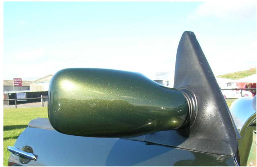
Replacement electric wing mirror which is finished in a colour to match the colour of the RV8 bodywork.
