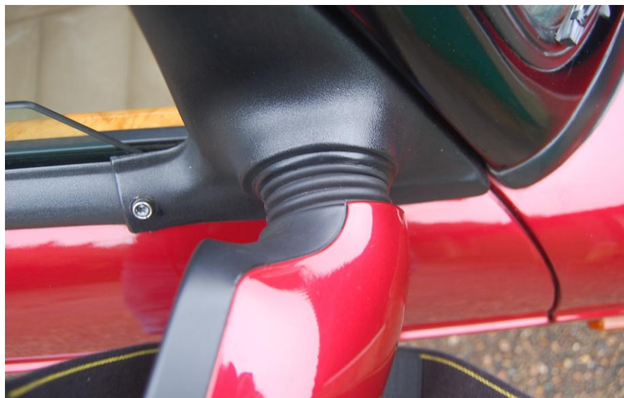
The replacement MGF wing mirror also includes a heating system – John Cumming has a switch below the dashboard to turn the wing mirror heater on and off as the MGF unit has the heater on permanently!
