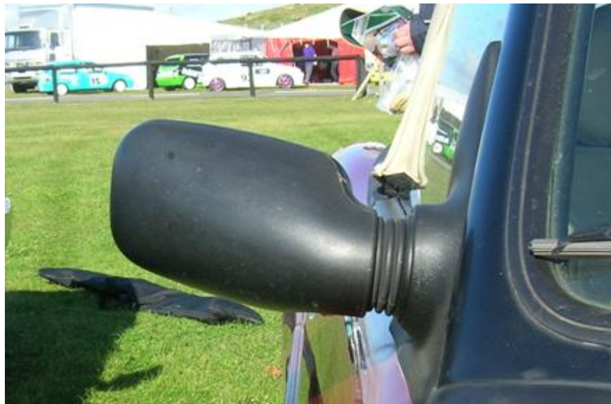
Original all black wing mirror fitted to an RV8 compared with the replacement MGF unit alongside.
