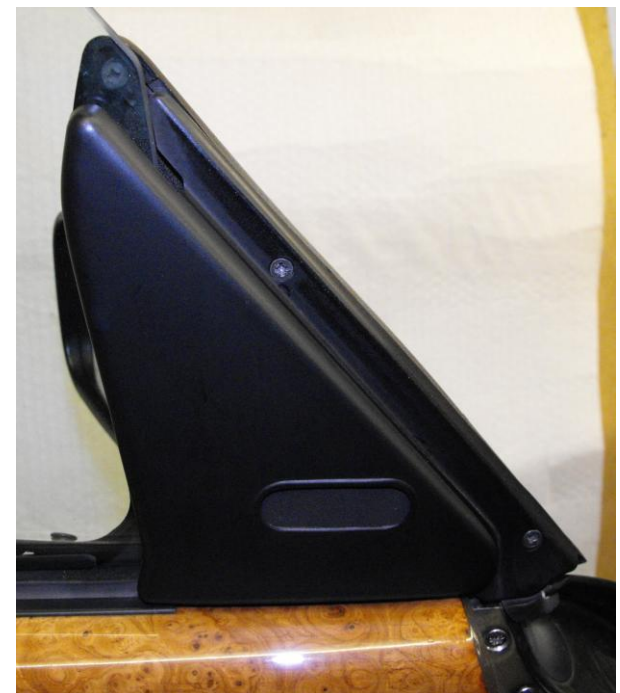
Replacement electric wing mirror which is finished in a colour to match the colour of the RV8 bodywork.
