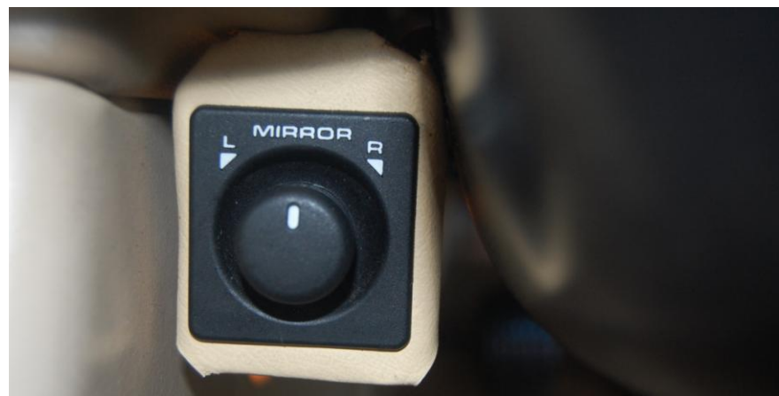
Knob on the electrically operated adjuster so the position of the wing mirror can be made remotely.
