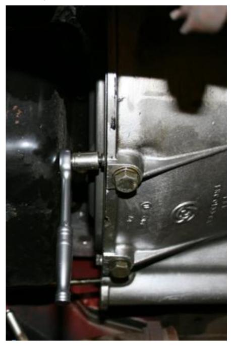
Nic Houslip provides a word of warning to those of you who use socket set ratchet handles that you need to push the spindle through and turn over to reverse the direction of operation.
