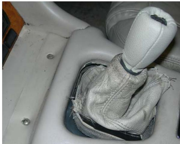
Richard recalled that he decided to tackle the worn gearknob and leather gaiter only to find that the bottom rubber gaiter had completely perished. He had a new gear knob, leather gaiter and rubber gaiter on order but wondered whether anyone had any tips on how to get new rubber gaiter over the "bulge" in the gear lever. At that stage he thought five minutes in hot water might make it more
