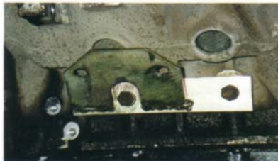
2-6-4-1 Cast engine mounts were not available so I fabricated this mounting and bolted it to the existing mounting holes in the block.
