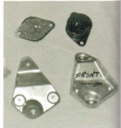
2-6-4-2 A recent development is the availability of cast replicas of the original V8 engine mountings, shown here. Clive Wheatley also has the special flexible V8 engine mountings, shown at the top of this picture. They are made from a different, firmer, rubber compound which is more resilient to heat.
