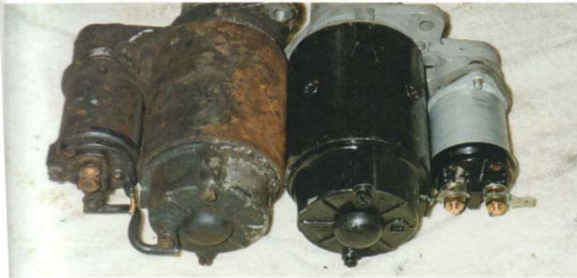
2-6-2 The original MGB V8 starter motor, seen here on the right, was a slightly shorter unit without a front connection to its solenoid. The SD1 starter (on the left) will suit most V8 conversions even if block-hugger exhaust manifolds are to be used. Take care with later Rover starters, particularly when the solenoid is mounted on the side of the motor, because you will then find it interferes with the MGB's chassis rails.
