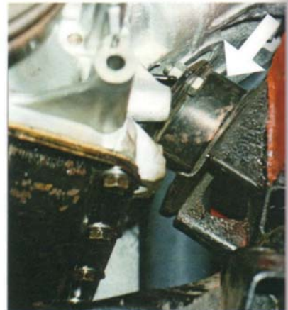
2-6-4-3 The flexible engine mount goes here. Note the hole in the rear of the fixed engine mounting bracket where, were this a LHD car, the steering shaft would pass. Note, too, the clearance between this rubber-bumper front crossmember and the sump of the SD1 engine – no problems here.
