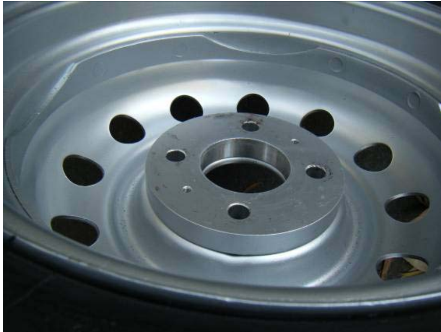
Above: aluminium spacer fitted to the Saab spacesaver wheel
