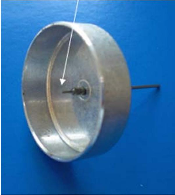
Bent dial spindle in the speedometer housing
