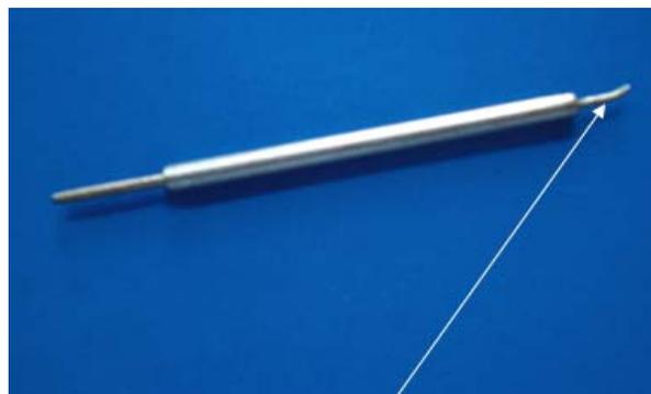
*Bent speedometer dial spindle. (Photo: Fa. Kienzle)*
