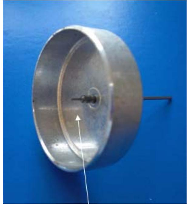
New dial spindle in the speedometer housing
