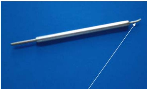
Damage to the spindle was sufficient to cause the speedometer to gyrate wildly.
