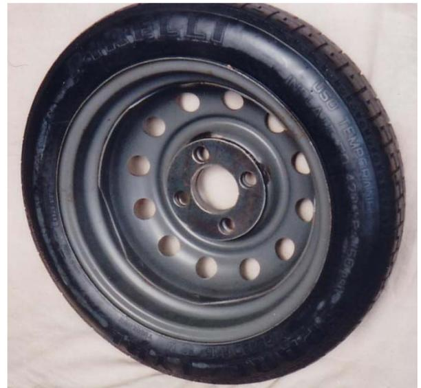
Inside face of the spacesaver with the spacer tack welded to the wheel. Note, spacer is made to fit over the hub of the axle. (Photo: John Bolt)
