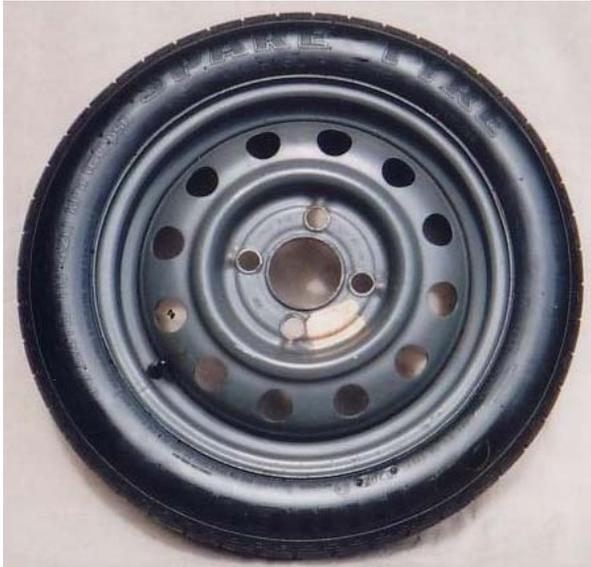
Outer face of the wheel with the four stud holes slightly countersunk to suit the tapered face of the wheel nuts. (Photo: John Bolt)
