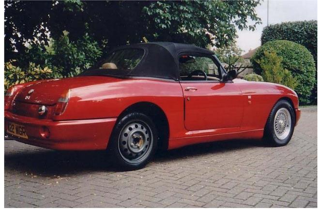
*Spacesaver fitted as a temporary rear wheel replacement. (Photo: John Bolt)*
