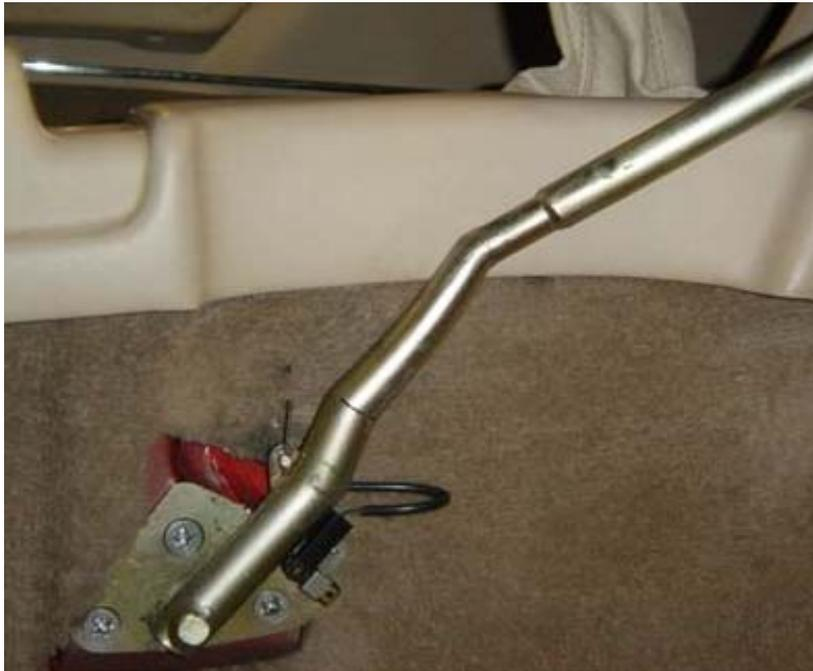
The modified handbrake lever refitted to the RV8 looks fine.
