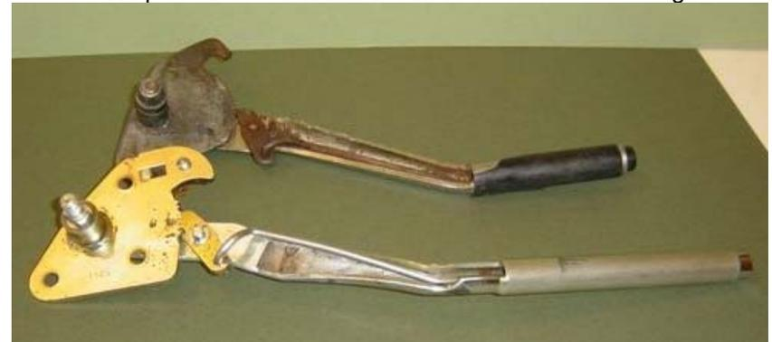
Comparison of an MGB handbrake lever (top) with the longer RV8 unit.
