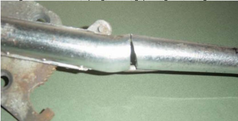
to cut right through the section. You can see in the second photo that a substantial portion of metal remains on the upper side of the shaft. Hugh used an old handbrake lever from an MGB to practice the cut to see how large the wedge shaped cut-out would need to be – 3/16 inch. He then refitted the handbrake and bent the shaft of the lever to the profile he wanted which included bending the head of the lever towards the driver's knee to clear the console - a quarter of an inch or so.
