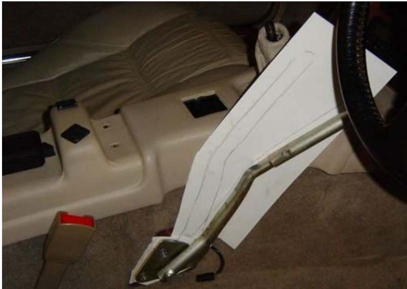
Using a sheet of stiff white card, Hugh marked out the position of the handbrake lever on his car before and after the re-profiling modification. The result is the head of the lever has been lowered by 5 inches.
