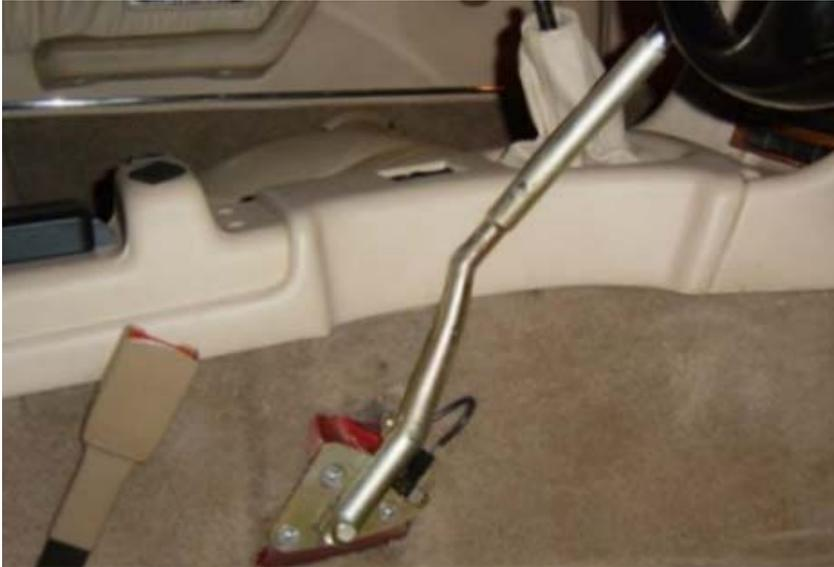
Hugh Boddington found the position of the handbrake grip in the off position on his RV8 was too high and uncomfortably close to the edge of the steering wheel. So he began thinking of how it might be modified so that it was lower. Note, the photo above has the driver's seat removed for access. As the handbrake ratchet and pawl stops the lever being parked at a lower position, Hugh decided the only way to lower the grip was to re-profile the handbrake lever.
