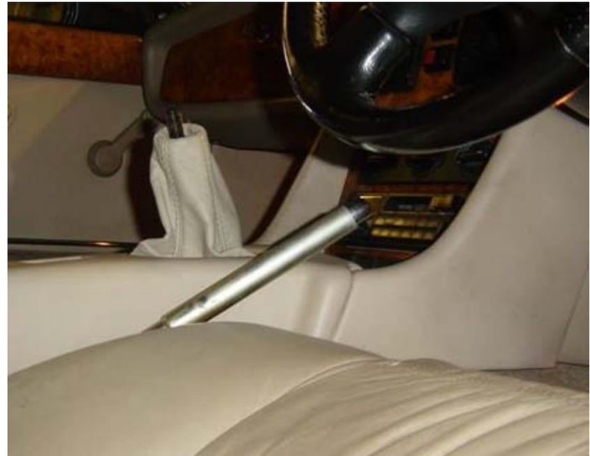
With the leather seat refitted, the modified handbrake lever clearly looks far better in its lower position, now well below the lower left hand edge of the steering wheel but comfortably above the edge of the console.
