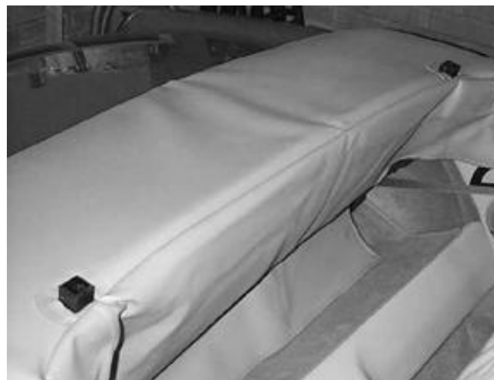
Figure 6: One of the finished holes, covered with the truncated circular finishing pieces, with the black plastic mounting block protruding.
