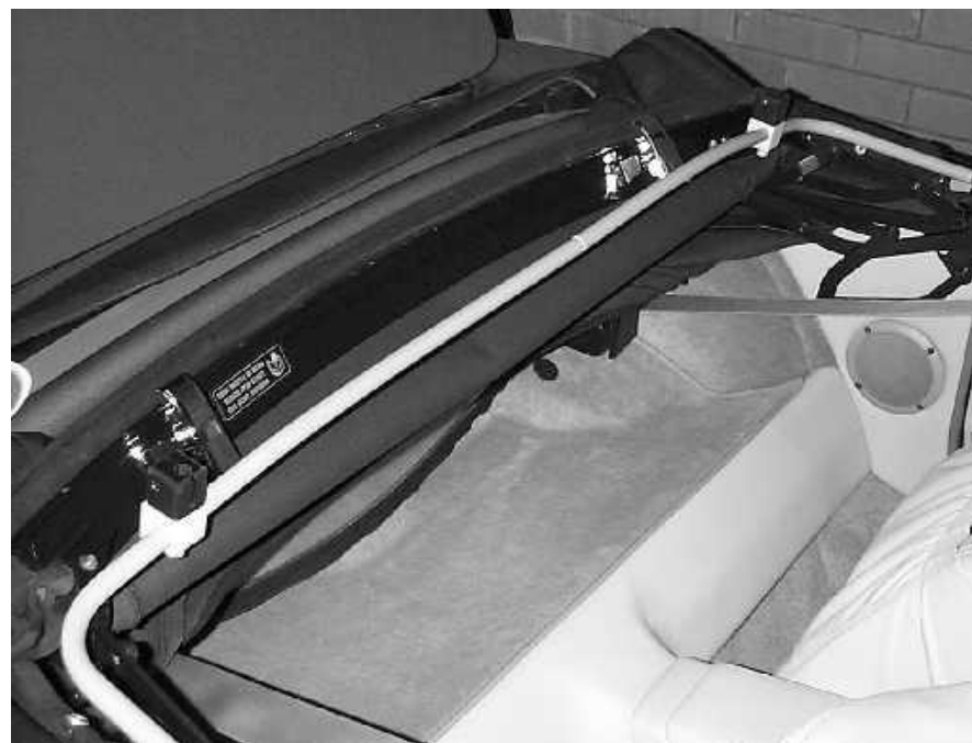
Figure 3: Half tonneau or hood cover support frame in position with the mounting blocks affixed. (The far one doesn't look too level in this photograph but the frame does go down a bit more when the cover is placed over it).
