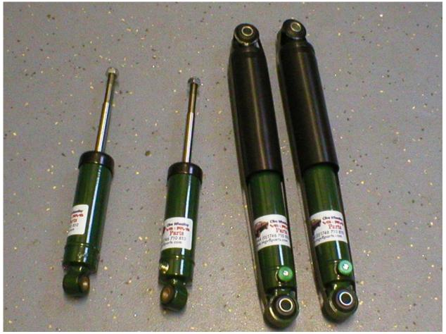
The second best rated mod was the fitting of SPAX shocks. 19 of the 25 respondents had fitted these. They are available from Clive Wheatley at £522 for a full set of four. The shocks were developed by SPAX specifically for the RV8 and offer complete flexibility with easy to change settings from 1 to 22. The settings can be changed without removing wheels by turning on full lock on the front or reaching around the tyre on the back. Very useful for track days.
