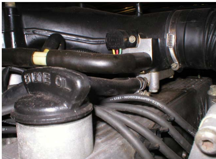
Hose (7) from the plenum cover plate (lower hose in the photo above)
