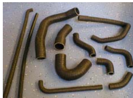
Set of replacement silicone water hoses for the RV8.
