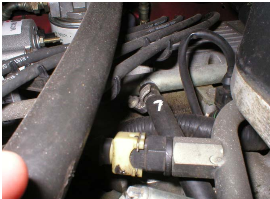
Hose (7) from the plenum cover connecting to the steel pipe/heater rail (13)
