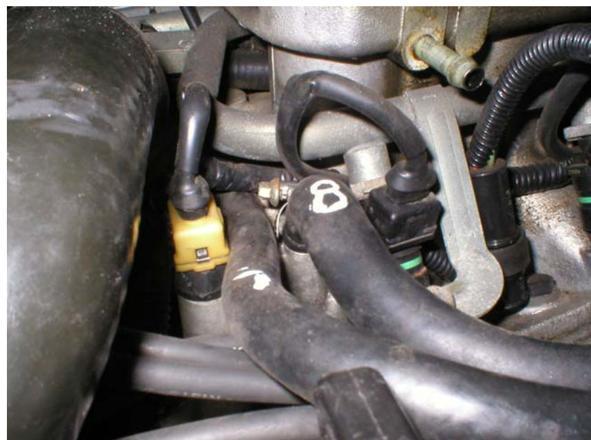
Hoses (7 and 8) with pipe above removed to show connection with plenum cover plate
